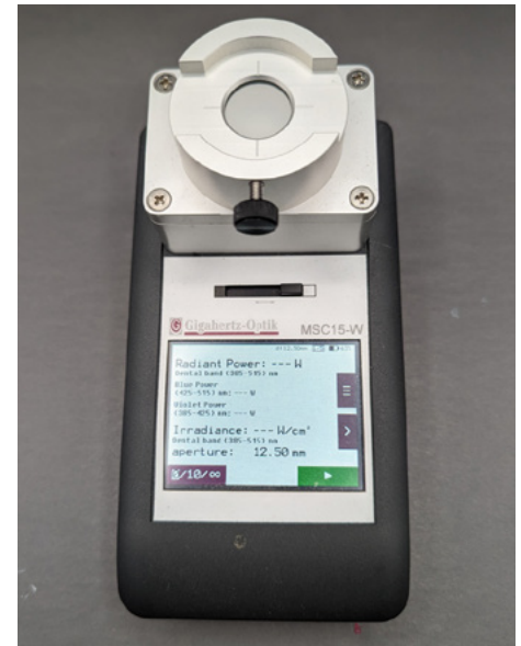
This is the Mini Gig (MSC15-W, Ultradent Products, Inc.) spectroradiometer with integrating sphere which accurately measures radiant power and spectral emission (wavelengths of light).
