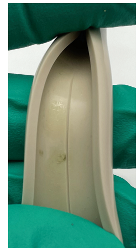
PowerScrub Vacuum Line Cleaner treated line.
