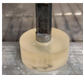
Cement is removed under load before continuing to cure in ~99% R.H. chamber for 10 minutes before testing or placed in water.
