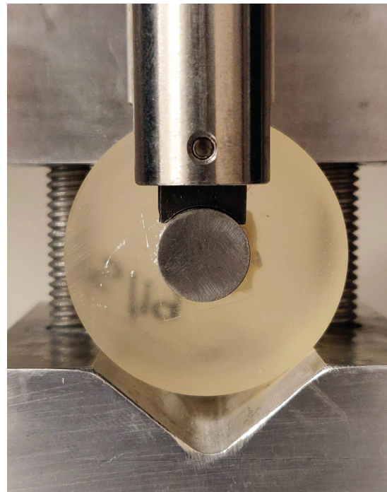
Shear bond test is conducted with 1 mm/min crosshead speed using an Instron model 5866.
