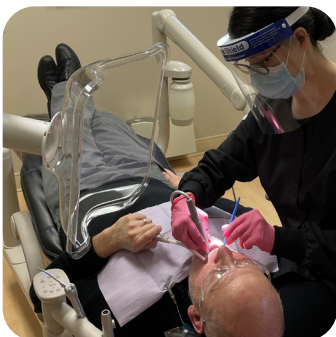
The Combi Hood can be integrated with Nederman FX 2 to allow for a larger source capture.
