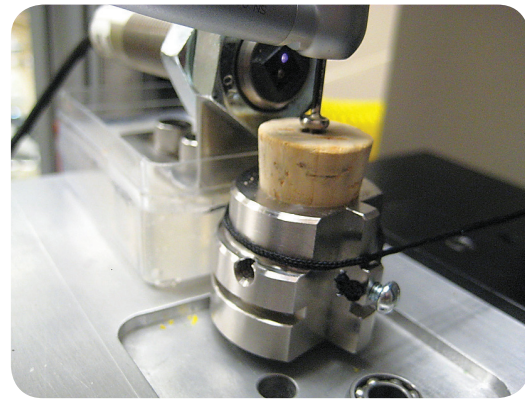
Close-up of torque sensor and speed sensor
