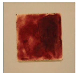
Figure 1: Representative untreated tile surface coated with 0.2 mL bacteria/blood suspension
