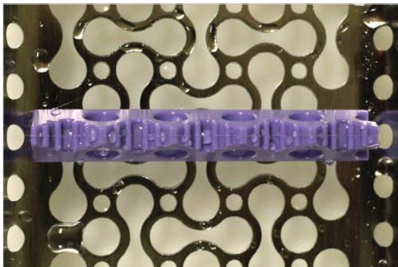
Figure 5. Appearance of Infinity cassette rails after cleaning of heavily soiled instruments. No evidence of any residual soil could be detected.
